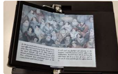
▲ 10.3" Print Color (E Ink Kaleido™) Foldable ePaper Display with built-in front light
