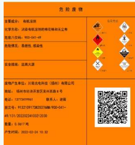
▲ Printing of hazardous waste QR code and attachment to the package to provide a unique anti-fake "ID" for each solid waste
