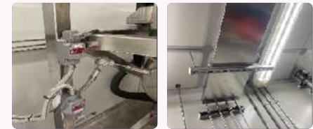
The tank positioning mechanism prevents equipment from starting to stir when it is not closed and not in the right position to reduce the risk of organic substances splashing/leaking and of objects drawn into or caught in the equipment
