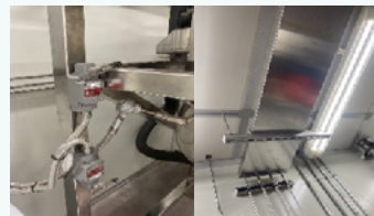
Implement a tank positioning mechanism to prevent operation if not securely positioned, reducing the risks of organic material splattering, leakage, and entanglement
