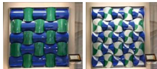
● A dynamic display column (Roller Coaster) using the E Ink Prism color programmable EPD.
