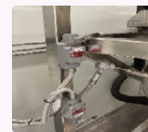
The tank positioning mechanism prevents equipment from starting to stir when it is not closed and not in the right position to reduce the risk of organic substances splashing/leaking and of objects drawn into or caught in the equipment
