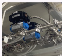
PLC control enables automatic exhaust when the pressure is too high and prevents the vacuum valve and exhaust valve from opening at the same time.
