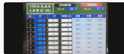
PLC's HMI system features timing and temperature control functions and enables immediate tripping and warning.
